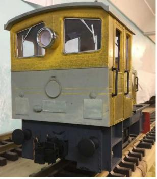
Buffer beams (plates) and Buffers were added.
